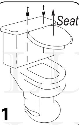
Remove the seat by unscrewing the seat.
