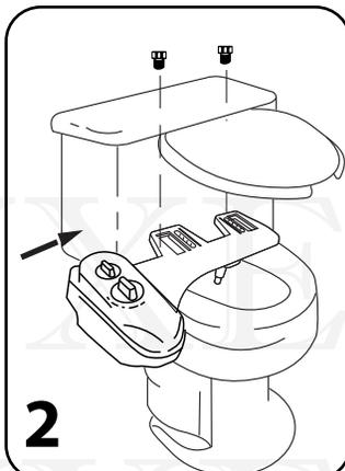
Place the bidet on the toilet. Align the seat coupling holes.
