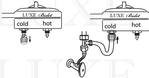
Connect the flexible tube to the cold water inlet on the bidet, tighten the wing nut on to it.
