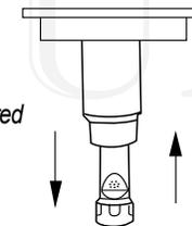
If your spray outlet hole is clogged for some reason, simply try to move spray outlet up and down for a few times manually.
